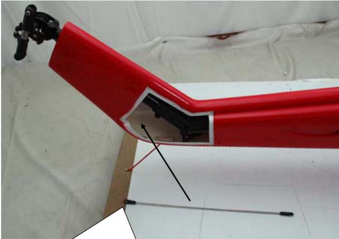
Connect the tail pushrod.
