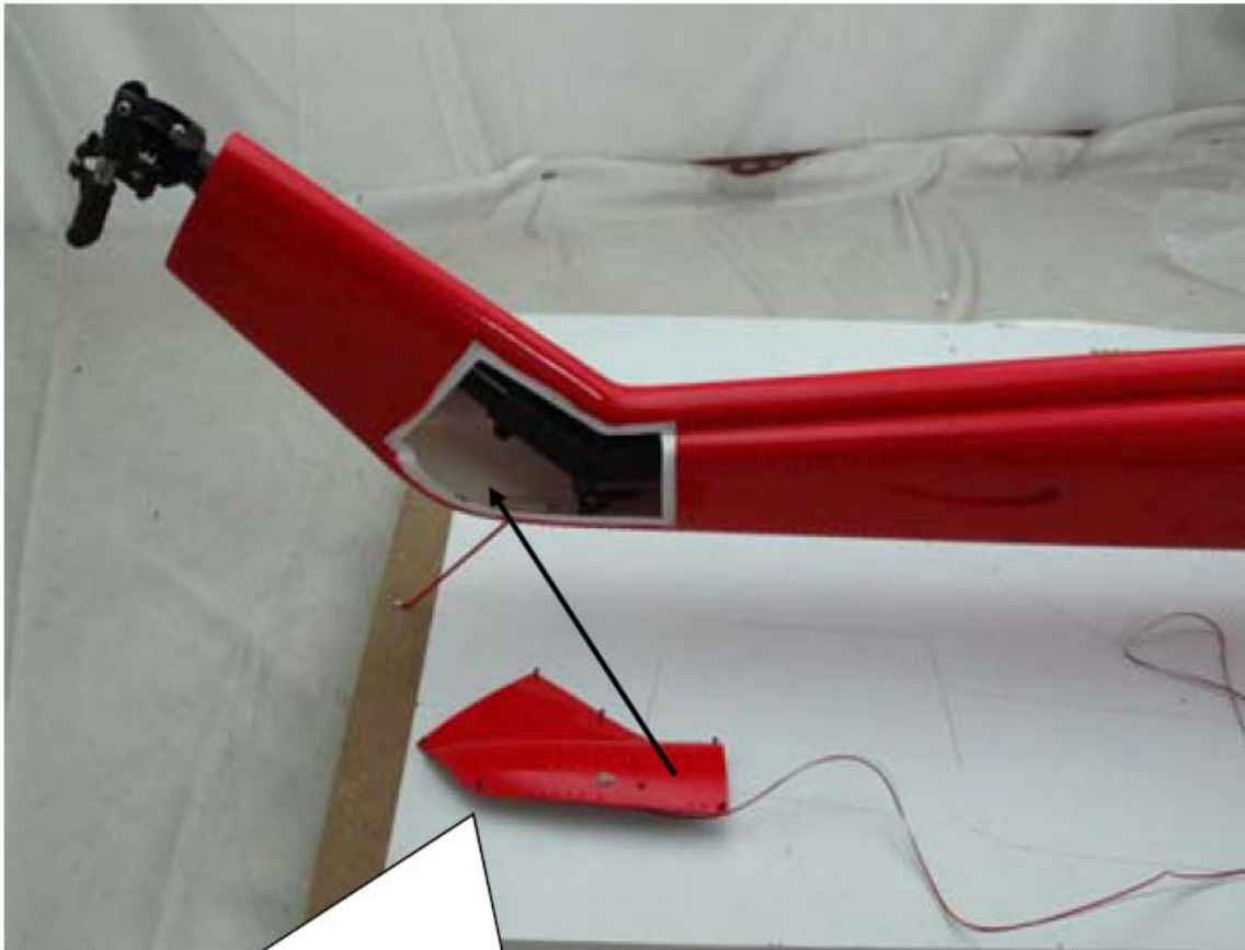
Attach the tail hatch again and route the light wires to the front.
