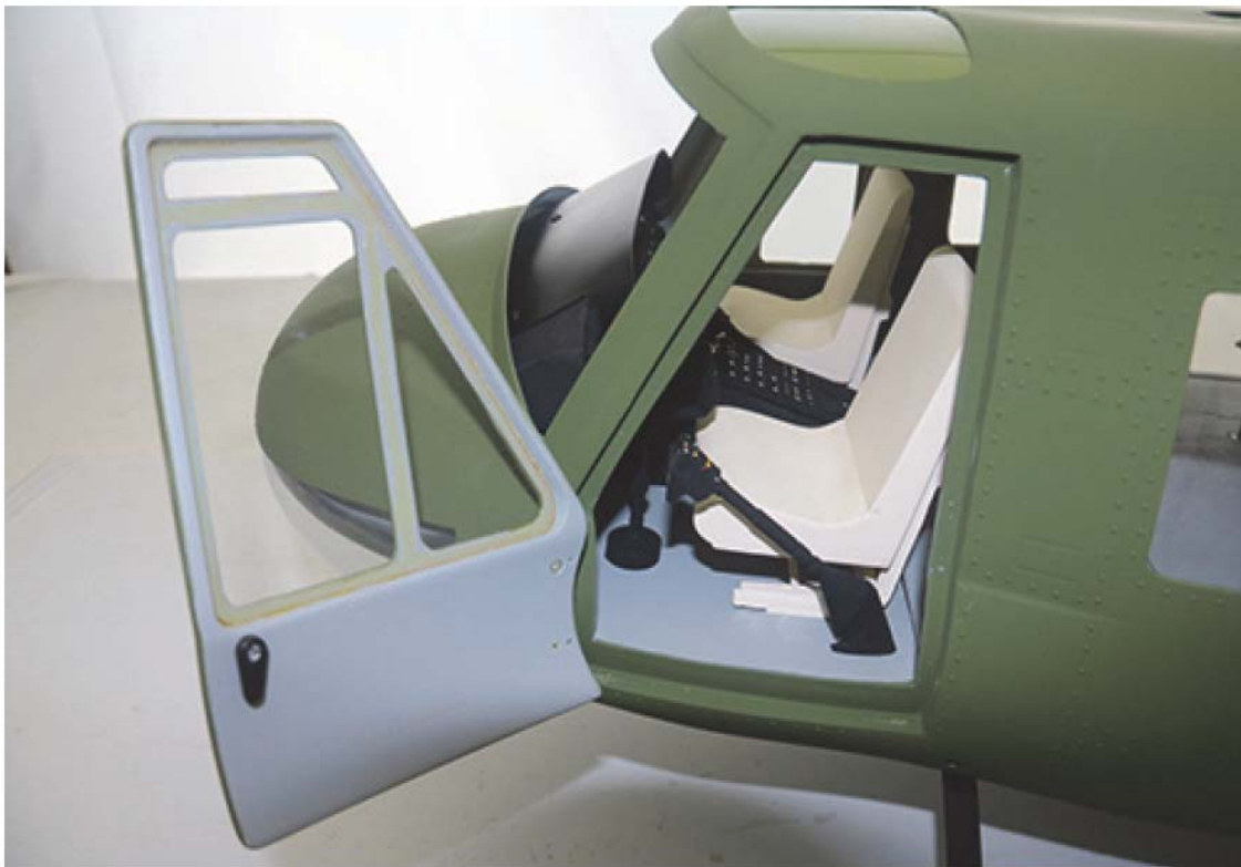
Finally mount both front seats 【69】
